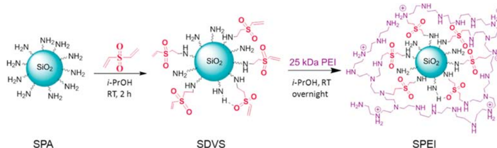
Scheme 1. Fabrication of SiO 2 -PEI NPs (SPEI NPs) via Coupling with DVS as a Linker
